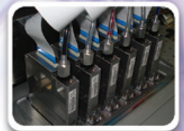
Japanese Original SII print head with automatic voltage control
